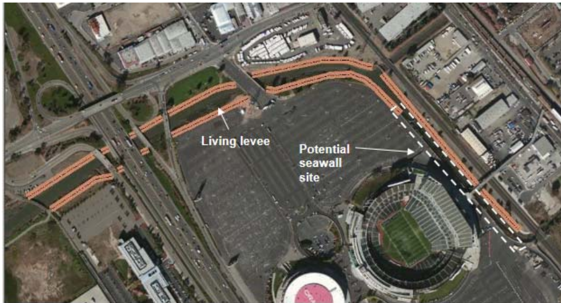
Figure 5: Layout and Footprint of a Living Levee System Along Damon Slough
