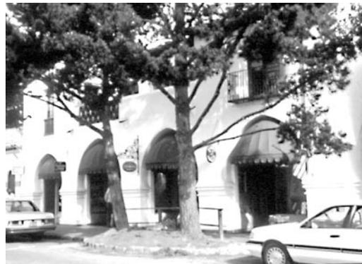
2.3.2 Relate awning shapes to window shapes and architectural features such as columns and pilasters. Use domed awnings over arched windows.
