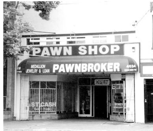
*Covered architectural detail / excessive signage and lighting / inappropriate bulkhead height and material / multiple security grilles and gates*
