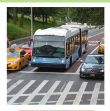
**Queue Jumps** increase the speed and reliability of bus service by giving buses a head start at signalized intersections.
