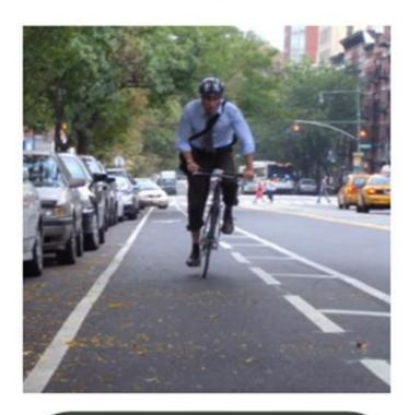
Buffered Bike Lanes provide additional separation between the travel lane and bicycle lane.
