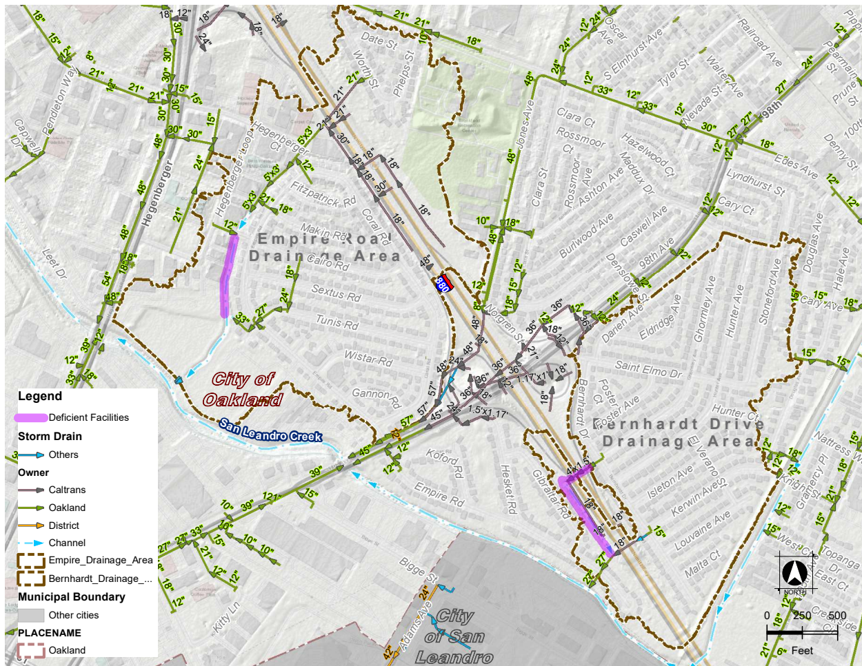
Figure 33 – Drainage Facilities Deficiency Map
