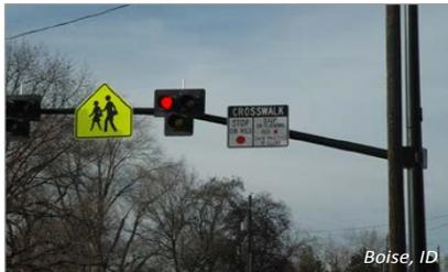
*A pedestrian hybrid beacon is a pedestrian activated display that is unlit when not in use. It begins with a yellow light alerting drivers to slow, and then displays a solid red light requiring drivers to remain stopped while pedestrians cross the street. Finally, the beacon shifts to flashing red lights to indicate motorists may proceed after pedestrians have completed their crossing.*
