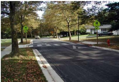
A pedestrian crossing or intersection area raised vertically to give motorists and pedestrians a better view of the crossing area. A raised crosswalk is essentially a speed table marked and signed for pedestrian crossing.
