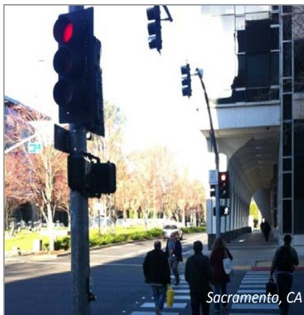
*A leading pedestrian interval gives pedestrians a 2-5 second head start before the concurrent vehicle phase turns green to allow pedestrians to enter and occupy the crosswalk before turning vehicles get there.*
