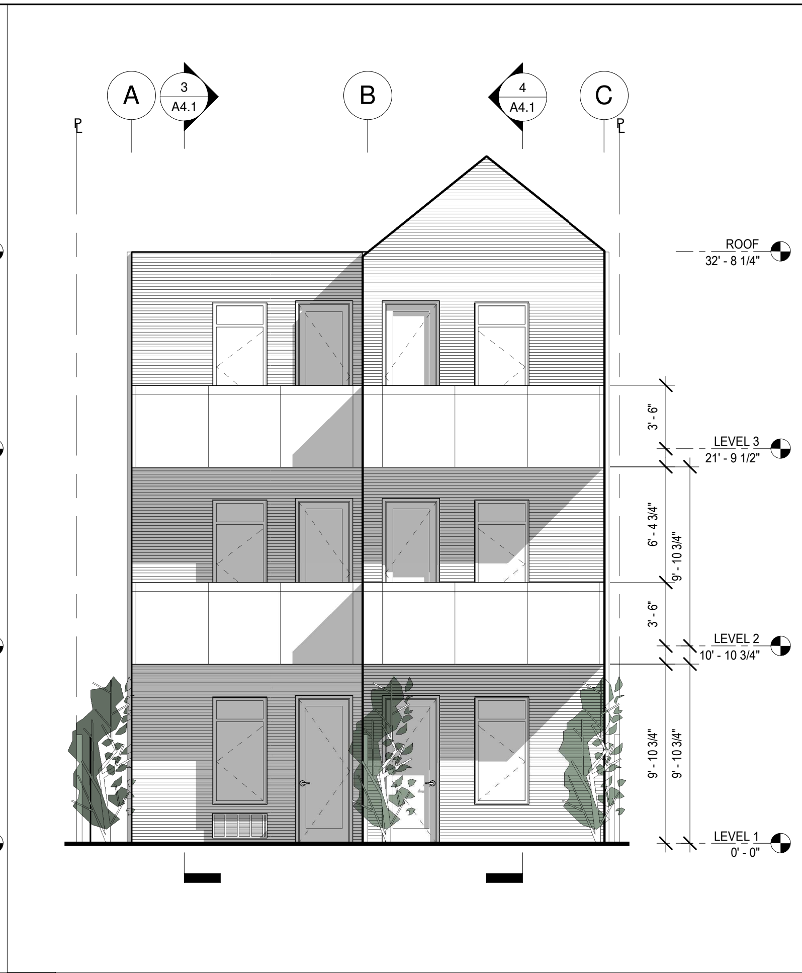
2 BUILDING ELEVATION - SOUTH SCALE: 3/16" = 1'-0"
