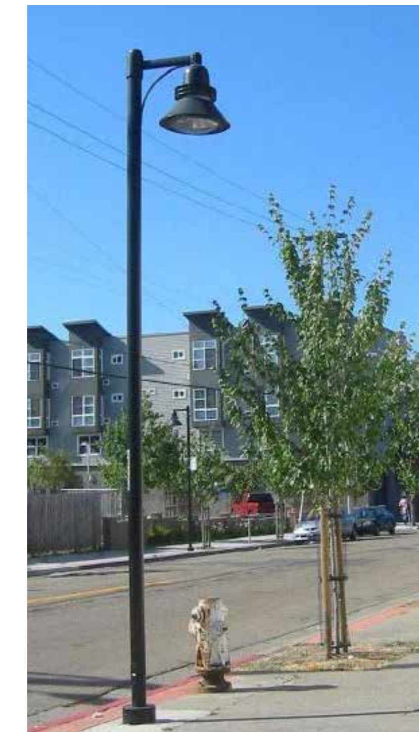
City Standard Lighting 'Universe' Luminaire and Pole, 20' Manufacturer: Architectural Area Lighting
