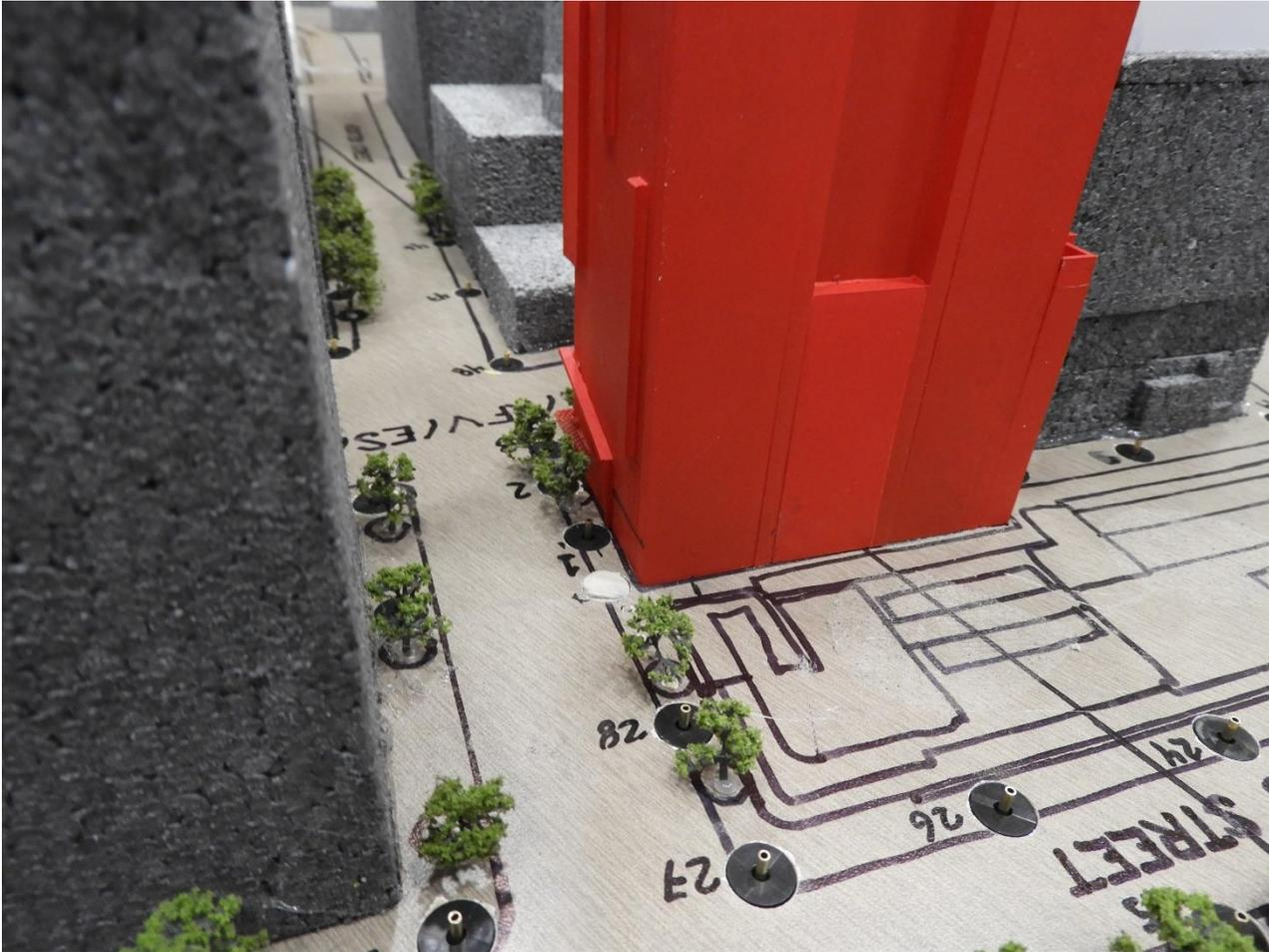
Image 2B: Wind Tunnel Study Model – Existing + Project Configuration
