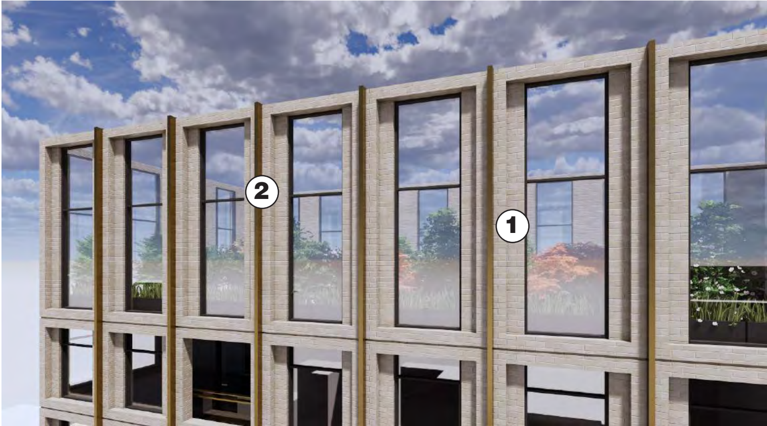
1. BEIGE BRICK VENEER ON PRECAST PANEL 2. BRONZE METAL FIN
