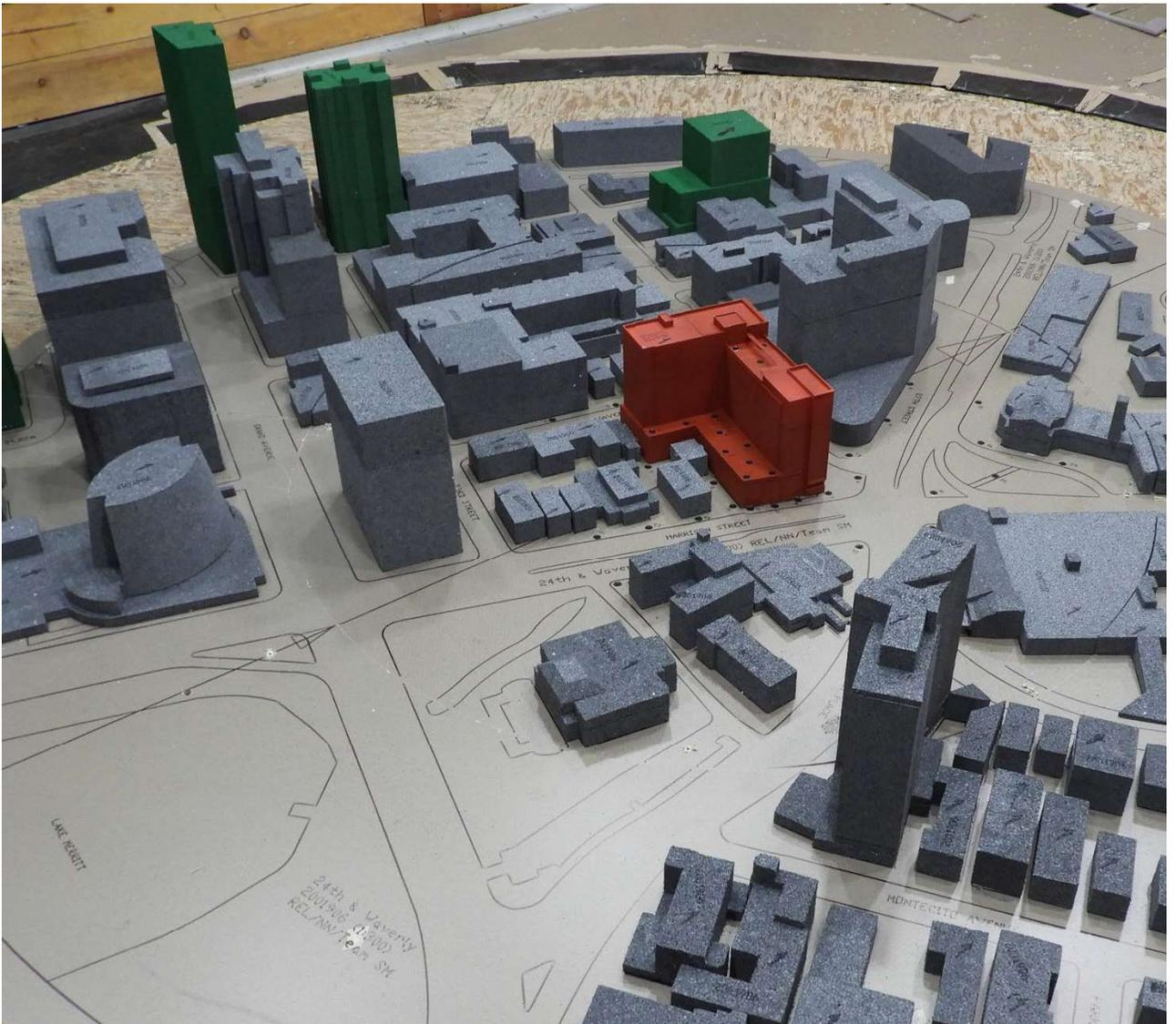
**Image 2C: Wind Tunnel Study Model – Project + Cumulative Configuration**
