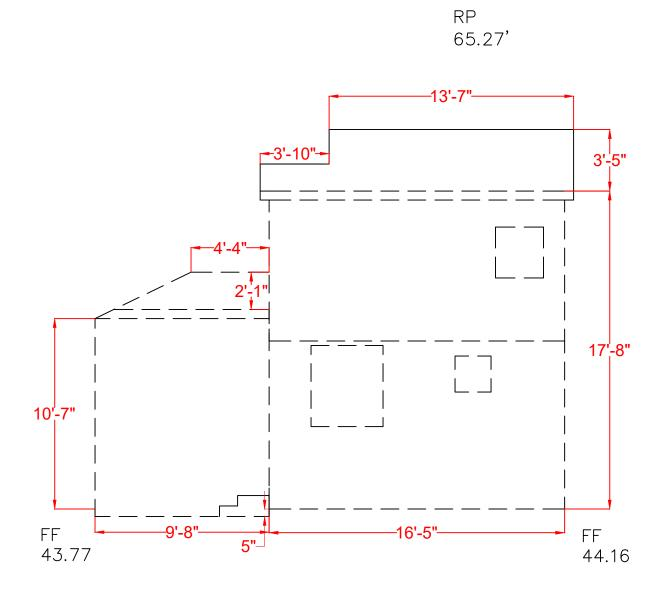
3 ACCESSORY BUILDING SIDE/WEST ELEVATION (TO BE DEMOLISHED) SCALE : 3/16":1'0"
