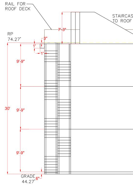
Bath )ne 94608 Bed/Four and 0 AND CA D Ses OAKL Φ -RAIL FOR ROOF DECK m STAIRCASES ownhou Four ----1'-----0 > 1031 62 ND ST 3'-3" MAX BUILDING HT RP 74.27**'** Eight 3RD\_FF 64.27' DESCRIPTION DATE 2ND\_FF 54.52' 1ST FF 44.77**'** GRADE 44.27' 1 NORTH/SIDE ELEVATION (PROPOSED) SCALE : 3/16":1'0" Door and Window Schedule **Townhouse North** and South DATE 04/25/2022 SHEET NO E-8
