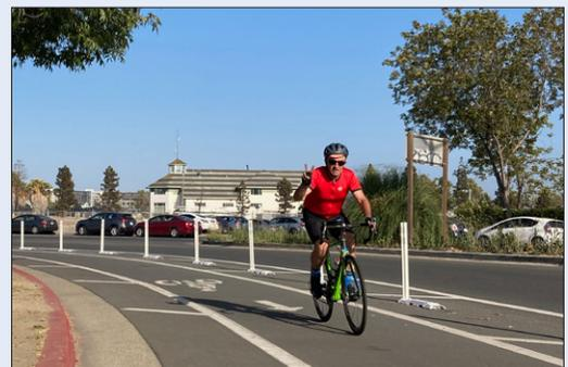
Vertical delineators separate bike lane from motor vehicles.
