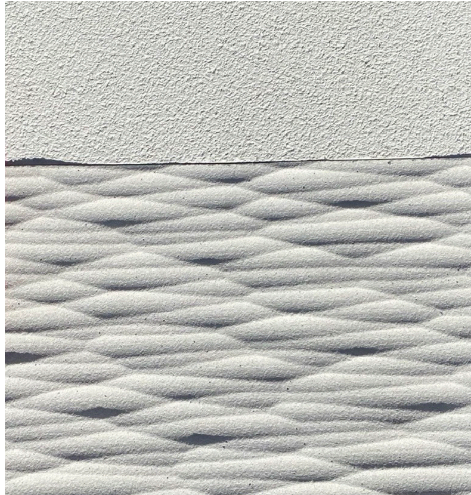
GFRC Samples top: no texture bottom: textured
