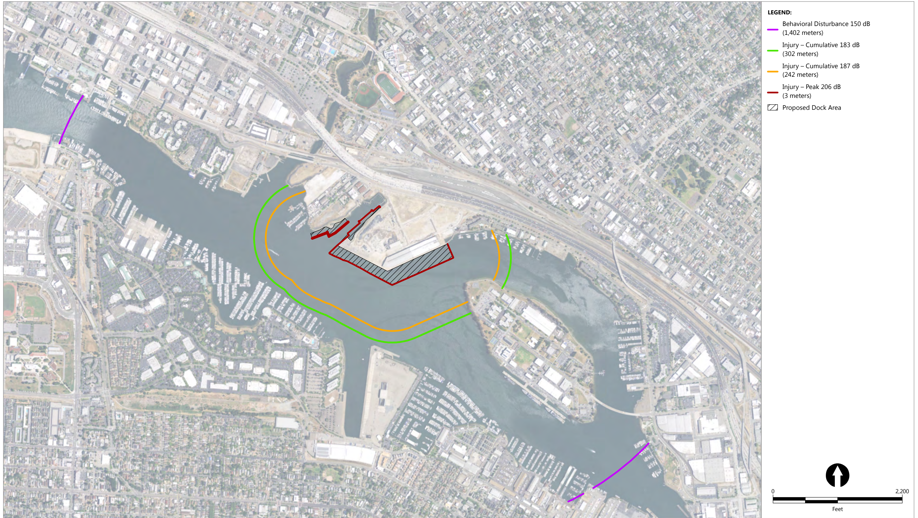
Figure 3 Fish Injury and Disturbance Zones for 18" Steel Piles Brooklyn Basin Development Project
