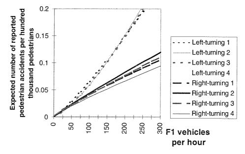
Fig. 7. Estimates of expected number of reported pedestrian accidents per pedestrian for  $F_2 = 50$  pedestrians per hour from the daily (1), a.m./p.m. (2), hourly (3) and 15-min (4) models for left- and right-turning vehicles.
