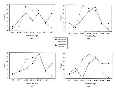
FIGURE 3 Percentage of crashes and exposure by pedestrian age group and roadway type at uncontrolled marked and unmarked crosswalks: (a) two-lane roads, marked crosswalks; (b) two-lane roads, unmarked crosswalks; (c) multilane roads. marked crosswalks: (d) multilane roads, unmarked crosswalks
