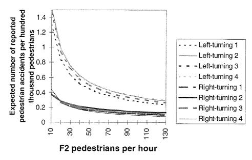
Fig. 6. Estimates of expected number of reported pedestrian accidents per pedestrian for  $F_1 = 500$  vehicles per hour from the daily (1), a.m./p.m. (2), hourly (3) and 15-min (4) models for left- and right-turning vehicles.
