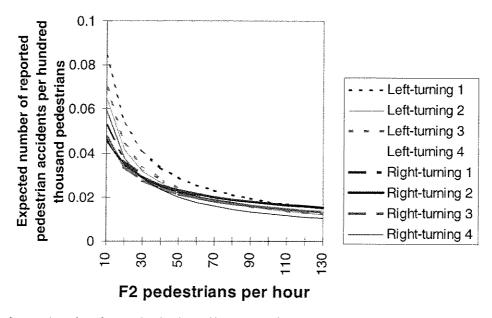
Fig. 5. Estimates of expected number of reported pedestrian accidents per day for  $F_1 = 50$  vehicles per hour from daily (1), a.m./p.m. (2), hourly (3) and 15-min (4) models for left- and right-turning vehicles.
