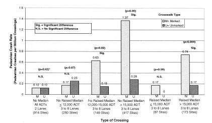
FIGURE 1 Pedestrian crash rate versus type of crossing (levels of significance between marked and unmarked crosswalks are based on binomial pedestrian crash modeling)
