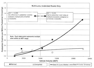
FIGURE 2 Pedestrian crash rates by traffic volume for multilane crossings with no raised medians—marked versus unmarked crosswalks.
